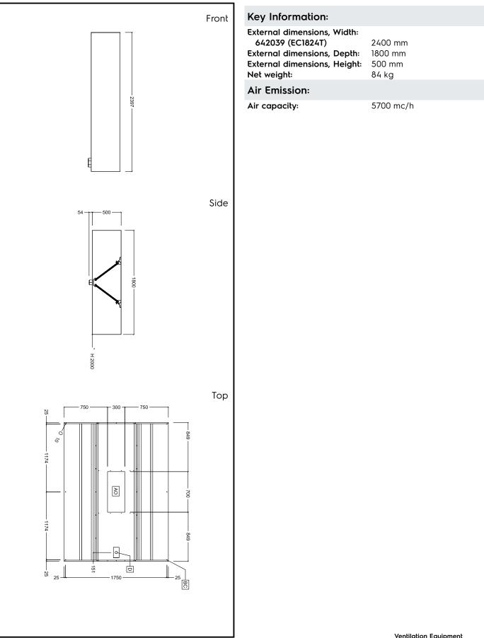
Ventilation Equipment 304 S/S Island Hood+Filters 2400X1800mm
